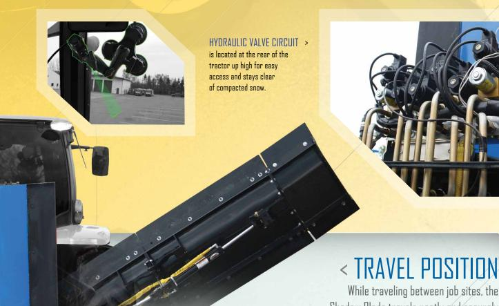
Shadow Blade travels neatly and securely behind the tractor.
